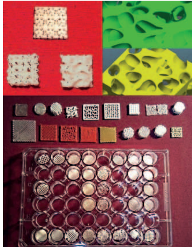
Figure 4. Gyroid structure-based 3D scaffolds, constructed with 3D Printer
