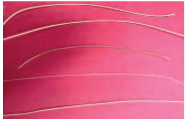
Figure 3. 1.75 mm diameter filaments, from PLA and PCL, enriched with metal complex compounds
