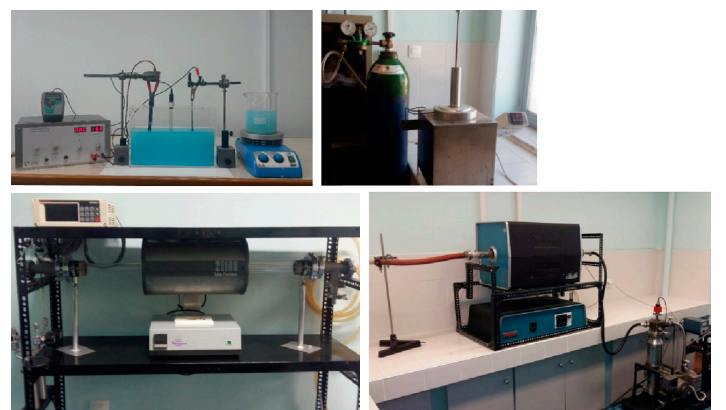
Figure 5 Material synthesis and growth using conditions of industrial production line, as Hot dip galvanizing, CVD methods, Electrodeposition and Melt-mixing. Application Fields regarding Synthesis and Characterization of Coatings and thin film technology, Thermoelectric Materials, Polymer Nanocomposites, Biomaterials-Bioceramics, Works of Art Preservation, Minerals & Gemstones, etc.
