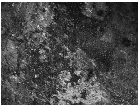
Figure 4 Images of the corroded samples (after 60h, 3.5%wt. NaCl solution at 35°C): (a) uncoated, (b) organic coating and (c) organic coating with AgNPs.
