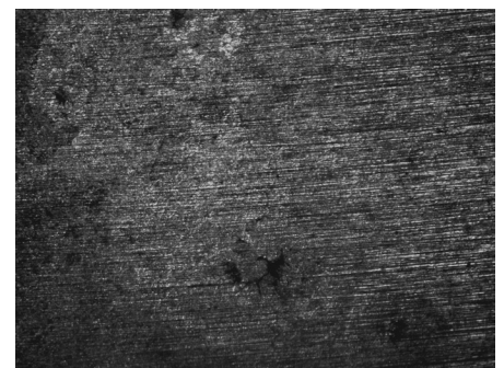
Figure 4 Images of the corroded samples (after 60h, 3.5%wt. NaCl solution at 35°C): (a) uncoated, (b) organic coating and (c) organic coating with AgNPs.
