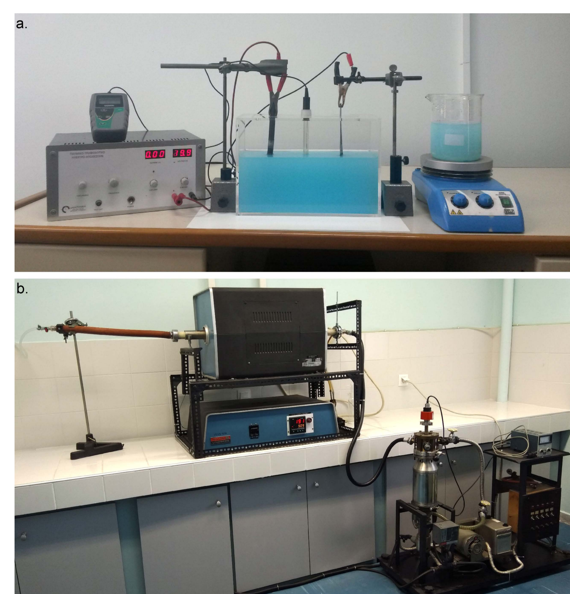
Figure 6: Material synthesis and growth using conditions of industrial production line, as Hot dip galvanizing, CVD methods, Electrodeposition and Melt-mixing. Application Fields regarding Synthesis and Characterization of Coatings and thin film technology, Thermoelectric Materials, Biomaterials-Bioceramics, etc. The images show (a) the Electrodeposition and (b) the CVD setup installed in the AMDE lab.
