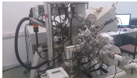
Back view of the system on the side of the Load lock chamber and of the Ar+ Ion Source.
