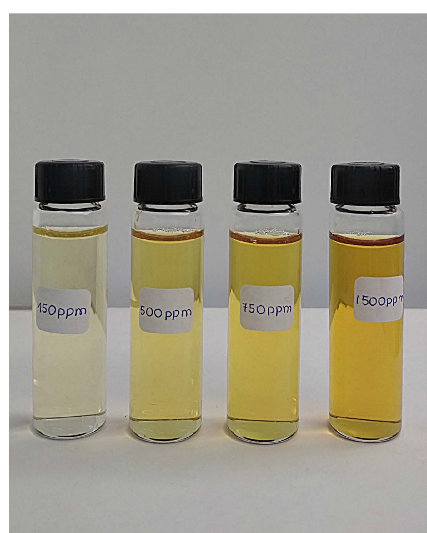
Figure 2 UV-Visible spectroscopy analysis of AgNPs suspensions at different concentrations.
