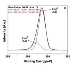
**4:** XRD (a) and XPS (b) measurements of polyethylene/graphene nanocomposite for pipe applications. Interplast-X.Op.Th. Laboratory collaboration aims to the extensive study and optimization of the materials, leading to higher performances of the final products.
