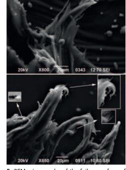
**5:** SEM micrographs of the failure surface of polyethylene/graphene nanocomposites, after tensile testing. Fractography analysis is a useful tool to determine the causes of failure and further improve the mechanical properties of the examined materials.
