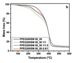
2: DSC (a) and TGA (b) measurements of unsaturated polyester resins derived from a biobased resource. CHIMAR-X.Op.Th. Laboratory aims to the extensive study and optimization of bio-based materials such as resins with similar or better performance than their petroleumbased counterparts.
