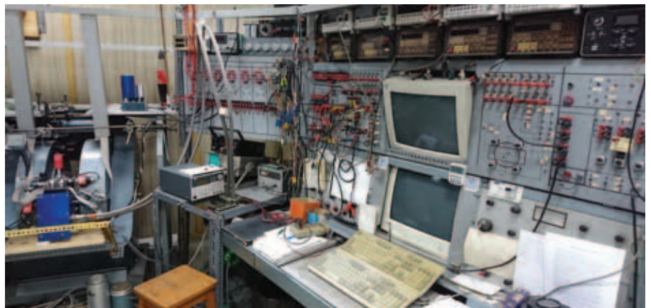
Figure 5 Van der Pauw and Hall measurements set-up for electrical characterization of materials in the temperature range of 10-330 K and magnetic fields up to 1.4 T.
