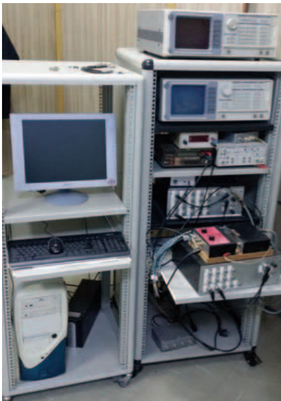
Figure 3 Computer controlled Low-Frequency Noise measurement system (1 Hz-100 kHz). It comprises two SR760 FFT spectrum analyzers, two SR570 low-noise current pre-amplifiers. All the critical stages are powered by NiMh batteries or are opto-isolated in order to reduce external noises and interference. The LFN technique allows for the characterization of carrier traps in semiconductor devices and materials.
