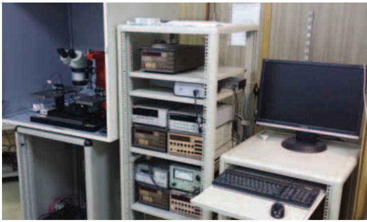
Figure 1 Computer-controlled system for I-V and C-V measurements, to fully characterize modern transistors or diodes. The system comprises voltage, current sources and arbitrary pulse generator, thus is capable for studying also Hot-Carrier effects (static & dynamic electrical stress)
